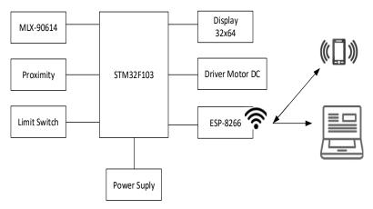
Gambar 2. Diagram blok rangcangan hardware
