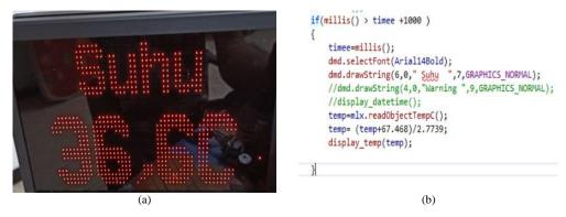
Gambar 6. (a) Display sensor suhu, (b) Kode program kalibrasi
