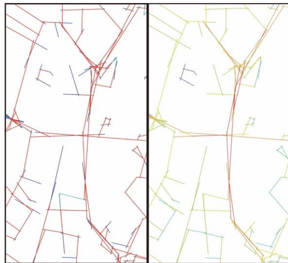
Figure 5. Connectivity on the segment on Kayutangan road (Left) and Integration on segment (Right) (Source: DepthMap Calculation)
