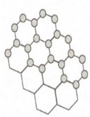
Figure 1. Configuration of pile installation with hexagon method (honeycomb)the test set-up
